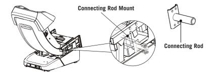
▶ There are brackets located at the top and bottom of the armrest to connect it to the main body. Attach the armrest to the top and bottom brackets. Secure with 4 screws on the bottom bracket, and 2 screws on the top bracket.
