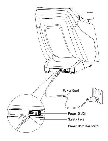
▶ After all parts are assembled, insert the Power Cord into the Power Socket, and then turn on the Power switch, press power on the remote control to start massage.
